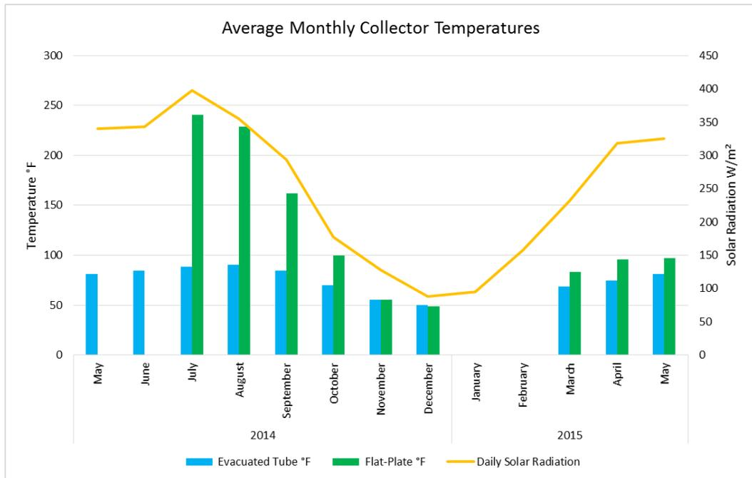
**Figure 10.** Average Monthly Collector Temperatures.
