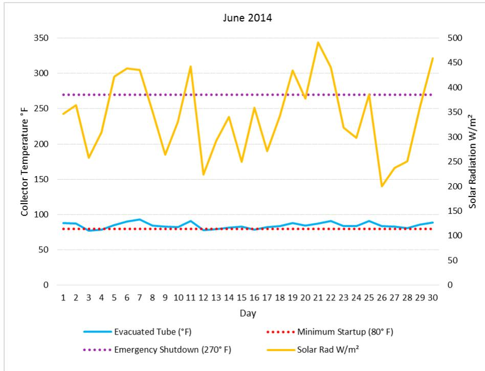
**Figure 12.** June 2014 Average Daily Collector Temperature and Solar Radiation.
