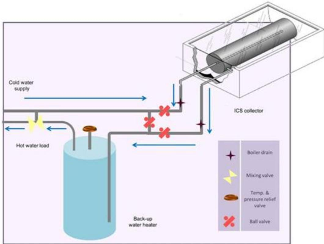
**Figure 8:** Integral Collector Storage. "Integral Collector Storage Solar Thermal System Layout." *Solar365*. N.p., n.d. Web. 19 July 2015.
