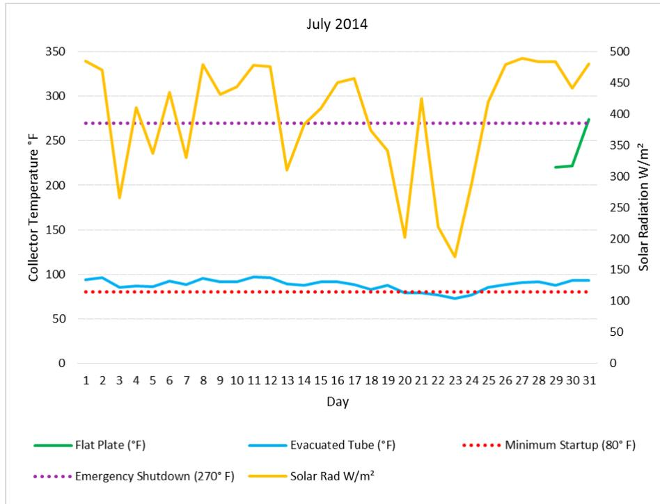
**Figure 13.** July 2014 Average Daily Collector Temperature and Solar Radiation.
