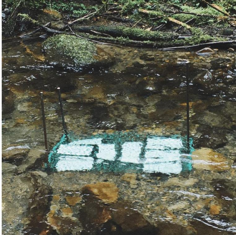
Figure 6. A periphytometer installed in the streambed.
