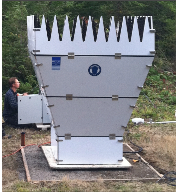
Figure 1: SoDAR installed at Primet
