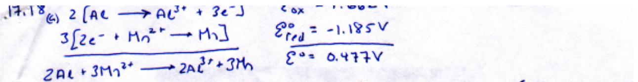
$$\Delta G^{\circ} = -nFE^{\circ} = -6 \text{ mole } e^- \times \frac{96485 C}{\text{mole } e^-} \times \frac{0.477 V}{C} = -2.76 \times 10^5 \text{ J spontaneous}$$
