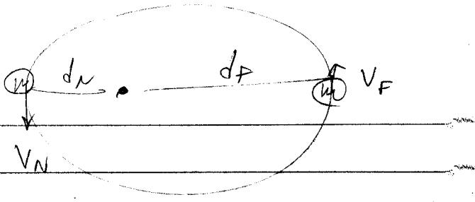
(a) Angular momentum is conserved, since no external torque operates:  $L_N = L_F$  where  $L = mv\mathbf{d}$
