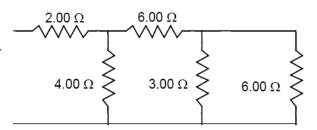
This equivalent resistor of  $6.00 \Omega$  is in parallel with the 3.00- $\Omega$  resistor, so
