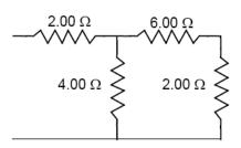
This new equivalent resistor of  $2.00~\Omega$  is in series with the 6.00-  $\Omega$  resistor, so  $R_S' = 8.00~\Omega$ .
