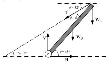
By applying the equilibrium conditions to the boom, we can determine the desired forces.
