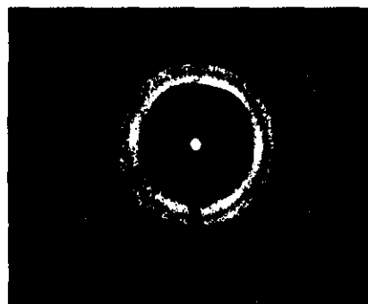
Fig. 5-10 Diffraction pattern produced by 0.0568-eV neutrons (de Broglie wavelength of 0.120 nm) and a target of polycrystalline copper. Note the similarity in the patterns produced by x rays, electrons, and neutrons. [Courtesy of C. G. Shull.]
