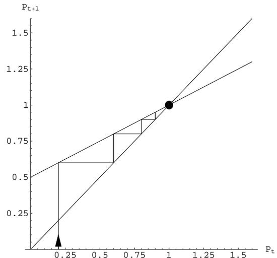
The equilibria occur where the function crosses the line  $y = x$ . These are indicated with dots on the graphs, with a solid dot being stable (cobwebs would approach it) and a circle being unstable (cobwebs would go away from it). When drawing cobwebs be sure to go up to the function first to get your output and then across to the line  $y = x$  to make your output the next input.
