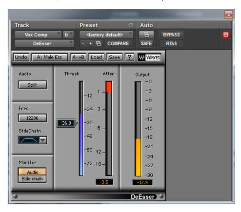
The letter "S" always sounds much louder than anyone wants it to when pronounced into a microphone. An accepted way to deal with this is to cut the amplitude of the "S" frequencies when those frequencies rise above a certain amplitude. This enables you to leave those frequencies present in between esses as opposed to removing them altogether throughout the whole track with equalization.
