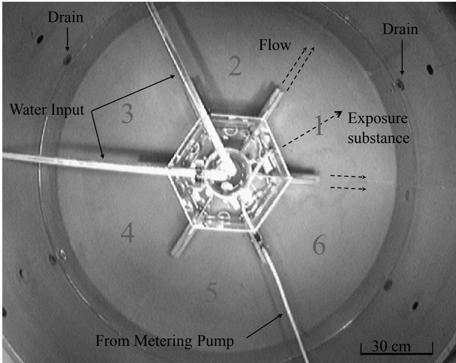
Figure 1. Overhead view of experimental chamber showing segment numbers (1-6). Double-dashed arrows indicate flow from dividers; single-dashed arrow indicates direction of flow of copper solution. Flow and drains are radially symmetrical. Copper solution was introduced in segment 1 only. Water input lines run over the top of the tank on the borders of segment 3.
