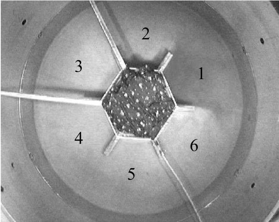
Figure 2. Overhead view of dye test showing containment of treatment water within the exposure segment (1). Distribution chambers are covered with fabric to eliminate reflections. Tank segments are numbered.
