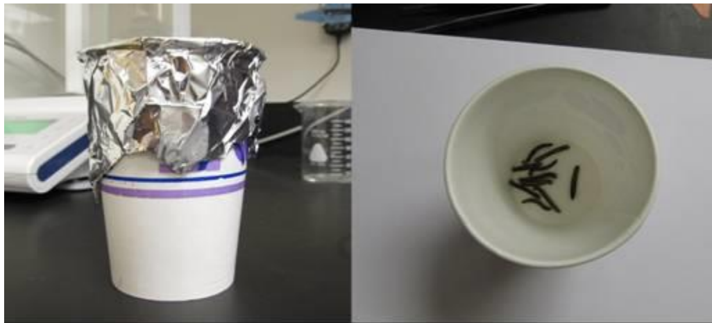
Figure 3.4 – Example of the sample cups used in this study. The image on the left shows the cup sealed with foil. This method of securing the sample larvae proved to be effective as no larvae escaped the cups during the study. The image on the right shows an aerial view of a cup after being taken out of the drying oven (foil removed).
