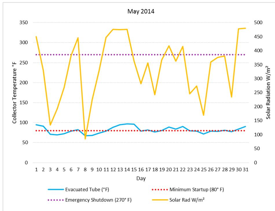
**Figure 11.** May 2014 Average Daily Collector Temperature and Solar Radiation.
