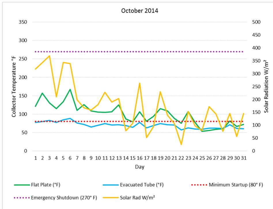
**Figure 16.** October 2014 Average Daily Collector Temperature and Solar Radiation.
