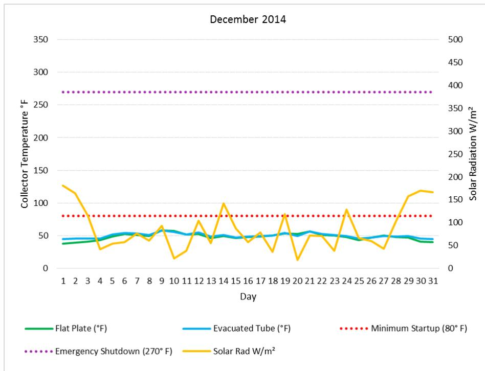
**Figure 18.** December 2014 Average Daily Collector Temperature and Solar Radiation.
