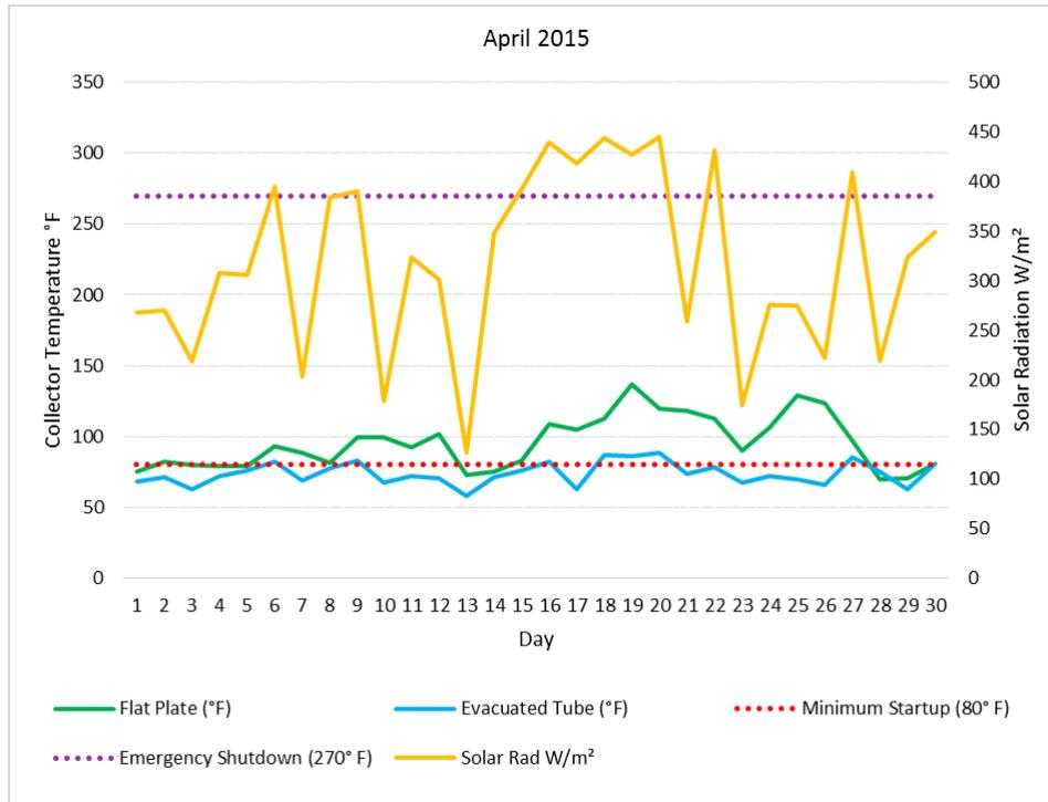
**Figure 20.** April 2015 Average Daily Collector Temperature and Solar Radiation.
