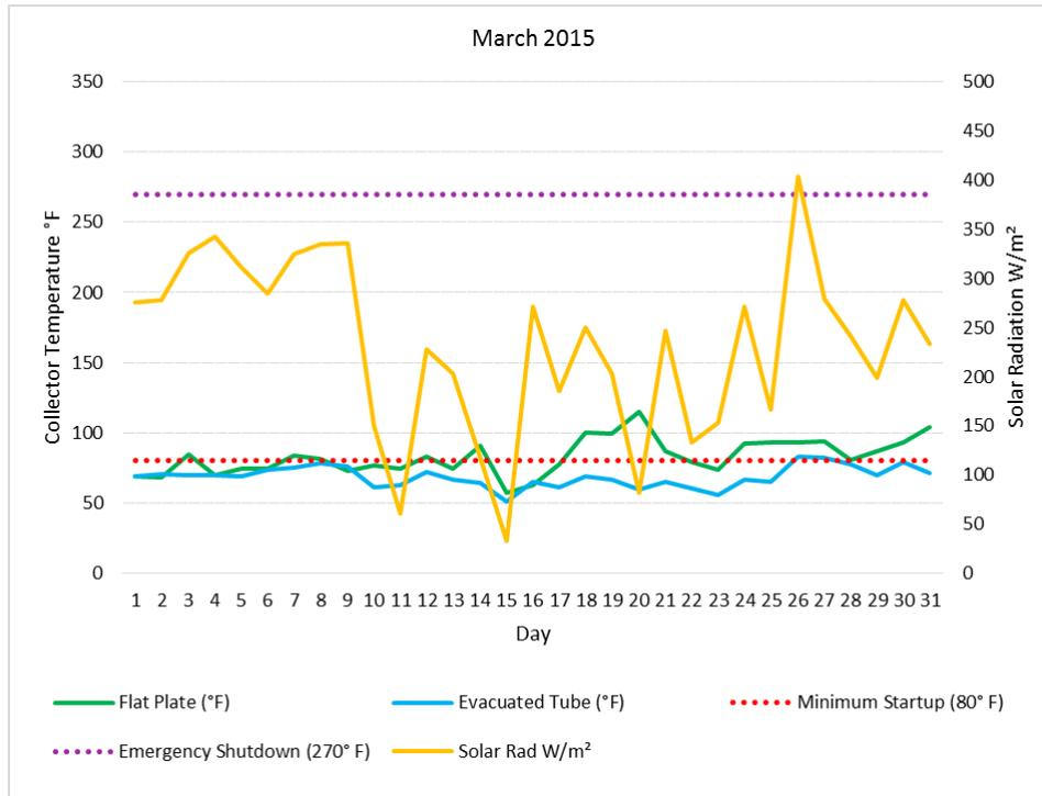
**Figure 19.** March 2015 Average Daily Collector Temperature and Solar Radiation.
