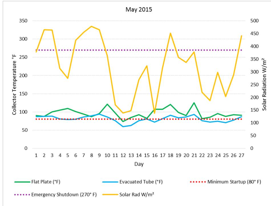
**Figure 21.** May 2015 Average Daily Collector Temperature and Solar Radiation.
