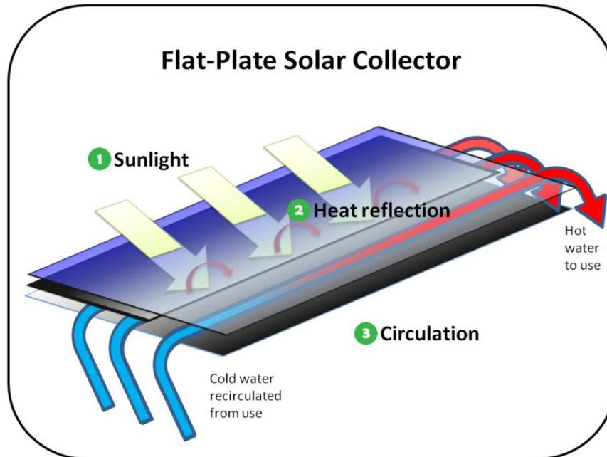
**Figure 3:** Flat Plate Collector. "Solar Heating and Cooling Technologies." *United States Environmental Protection Agency*. Environmental Protection Agency, 8 May 2015. Web. 11 Aug. 2015.
