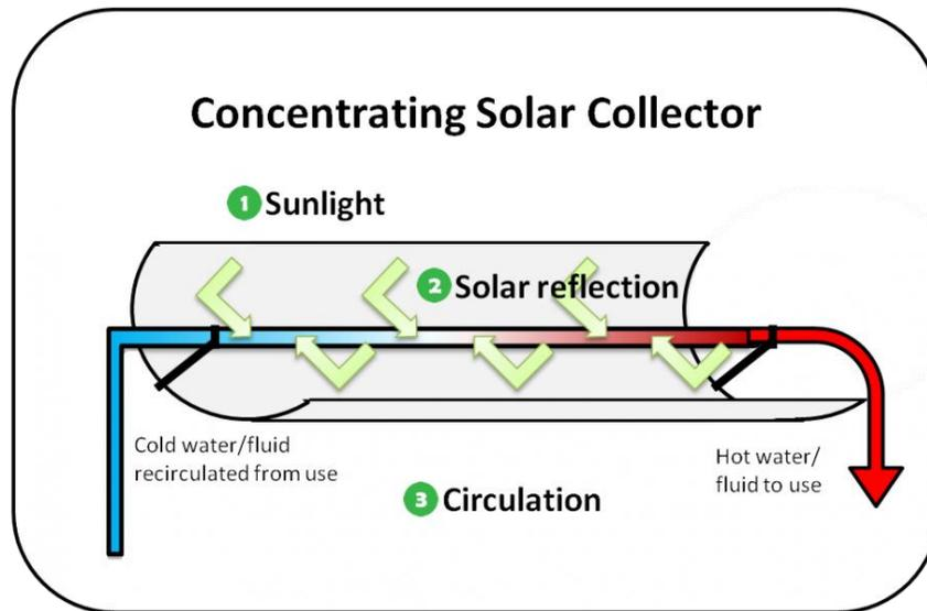
**Figure 5:** Concentrating Solar Collector. "Solar Heating and Cooling Technologies" *United States Environmental Protection Agency*. Environmental Protection Agency, 8 May 2015. Web. 11 Aug. 2015.
