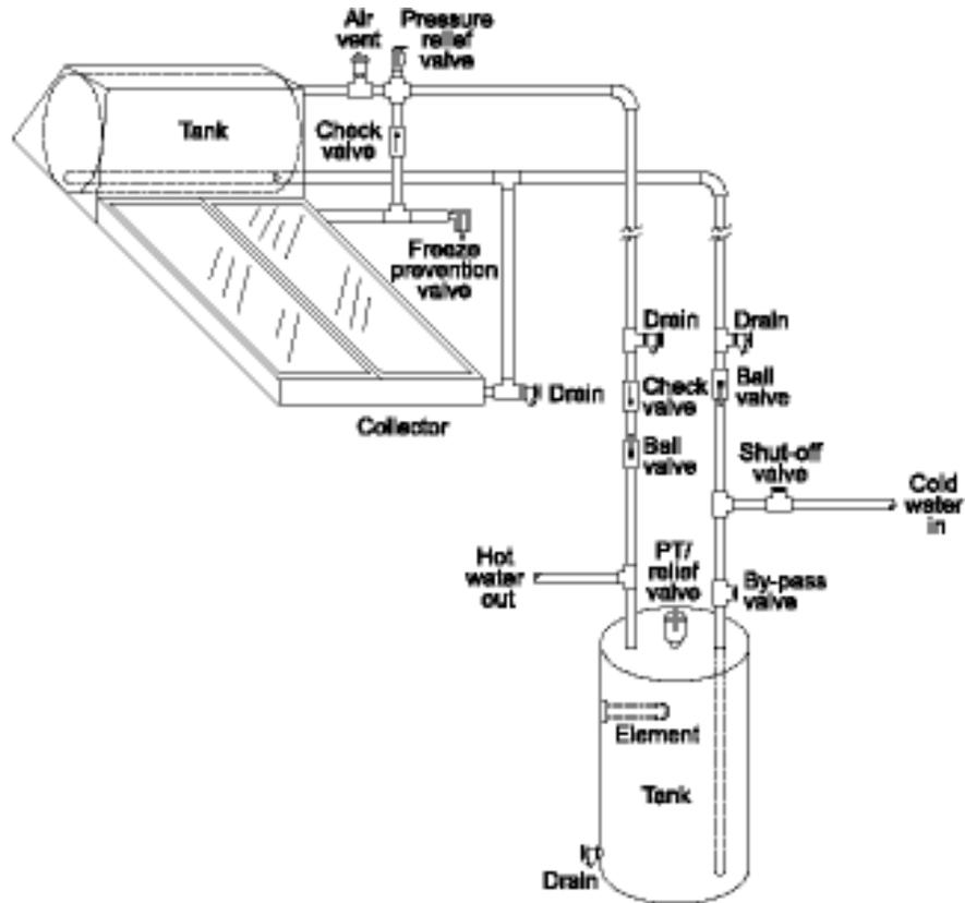
**Figure 7:** Thermosyphon System. “System Types.” *Florida Solar Energy Center*. N.p., n.d. Web. 2 May 2015.
