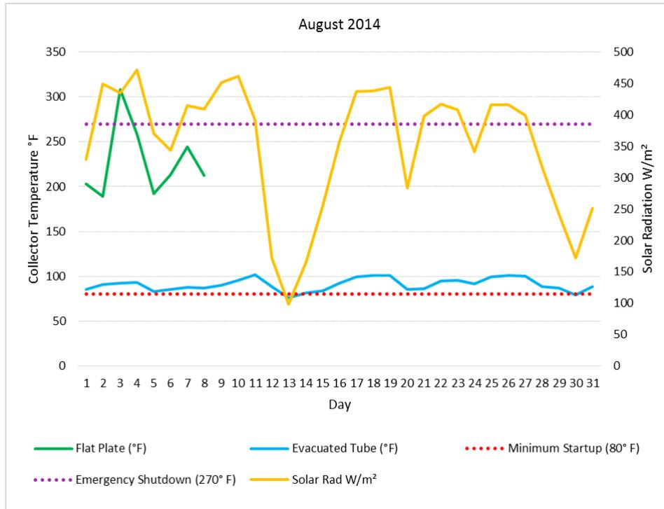
**Figure 14.** August 2014 Average Daily Collector Temperature and Solar Radiation.
