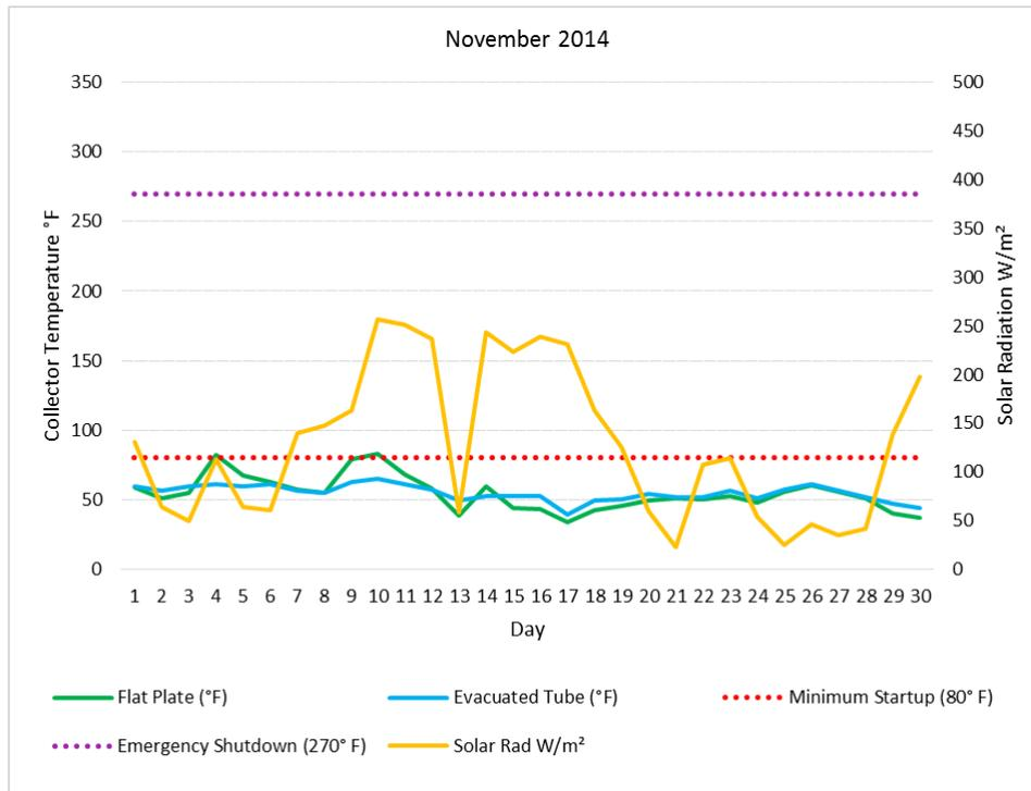
**Figure 17.** November 2014 Average Daily Collector Temperature and Solar Radiation.
