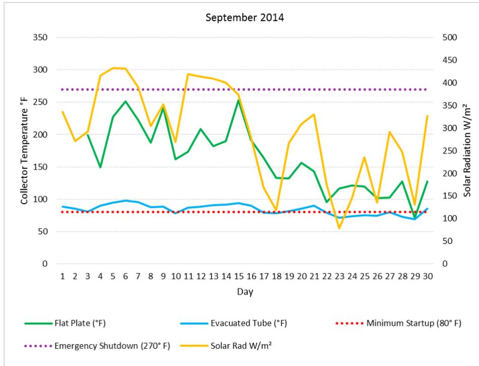
**Figure 15.** September 2014 Average Daily Collector Temperature and Solar Radiation.
