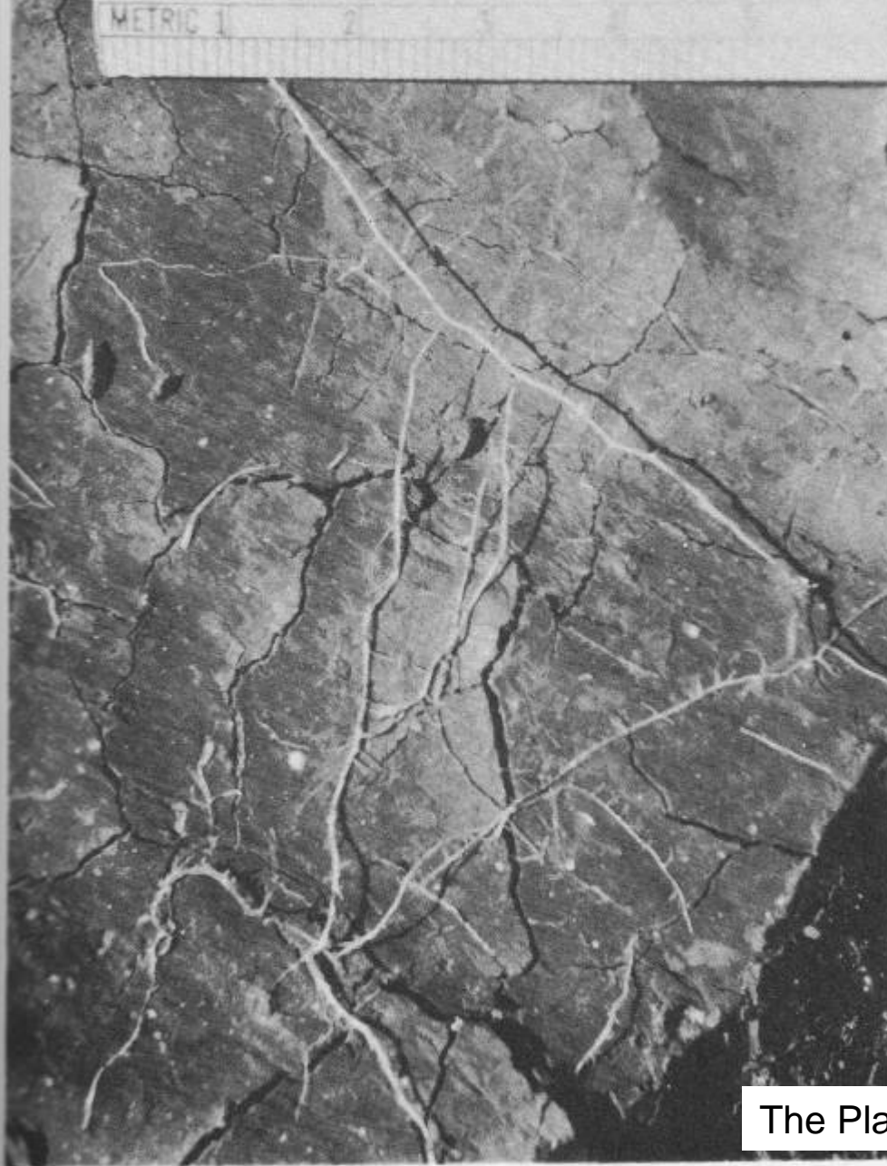
Fig. 11.6. Plant roots located in a vertical shrinkage crack of Houston Black clay. Note that the roots apparently were unable to readily penetrate the vertical face of the crack. (Photograph courtesy of E. Burnett)
