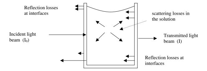
The diode array spectrometer is based on Beer-Lambert's law. Beer-Lambert's law relates the absorbance of light passing through a medium (a solution, in this case) to the path length and concentration as follows.
