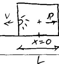
(a)  $P_{\text{light}} = \frac{E}{c} = -(P_{\text{box}} = M_1 V) \rightarrow V = \frac{E}{M c} = \text{recoil speed of box}$
