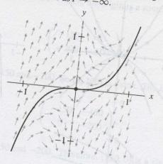
(g) Solutions tend away from the origin along the y-axis in both systems. In the nonlinear system, solutions approach the origin along the curve  $y = x^3$  which is tangent to the x-axis. For the linearized system, solutions tend to the origin along the x-axis. Near the origin, the phase portraits
