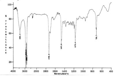
The IR spectrometer outputs the spectrum as wavenumbers, C in cm<sup>-1</sup> instead of frequency in Hertz. In this case the wavenumber is simply the reciprocal of the wavelength  $v' = \frac{1}{\lambda}$ .
